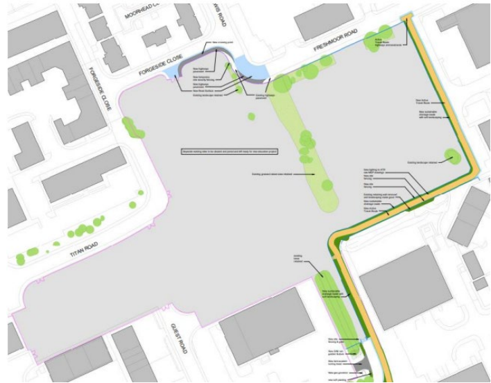
Figure 3: Proposed site layout of the enabling works application (22/02308/FUL) with active travel route in yellow, pavement highway works to the north and the turning head to the south.
